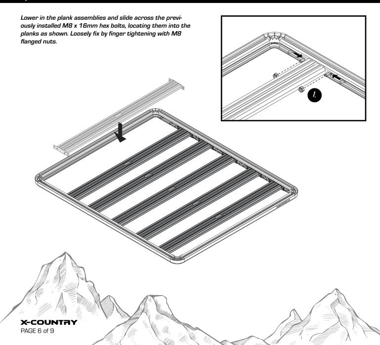
Position the installed planks into their correct positions.
